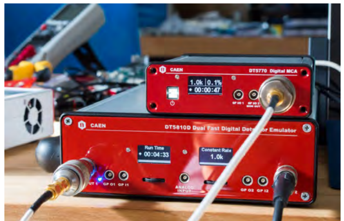
A simple emulation and evaluation setup: CAEN DT5810 and DT5770 single input digital MCA.
