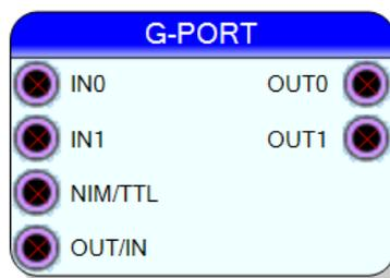
In order to use one G-PORT as input and the other as OUTPUT, set the OUT/IN pin as OUTPUT (Low) and force LOW the INx pin of the G-PORT so we configure it as following
