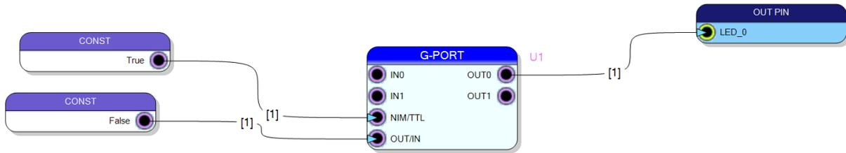
Then we peek from board pin the Gate and Delay block. The tool ask as to specify which of the channel of the G&D use. Pay attention to do not use multiple time the same channel. There are 32 channels and user must care to use each one for no more than one IN/OUT pair
