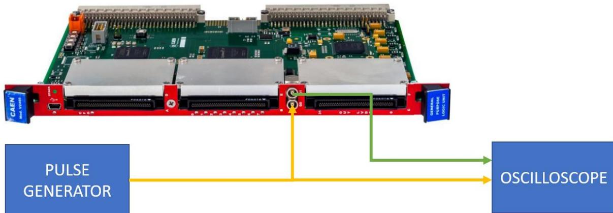
Set the signal generator to generate a square wave 1KHz, TTL, 50% duty cycle
